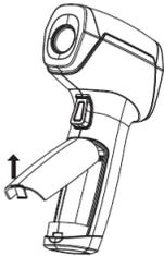
This product uses 2 AA batteries. Remove the battery cover and place the batteries according to the polarity diagram in the battery compartment.
