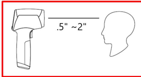
4. Pull the "Power/Measure" trigger and release. The thermometer beeps when the reading is complete. The temperature displays in the LCD Viewing window.
